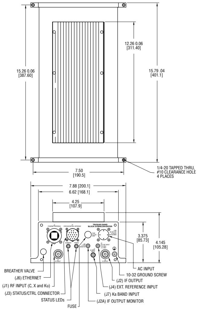
Note: Dimensions shown are in inches and those shown in brackets [ ] are in millimeters.
