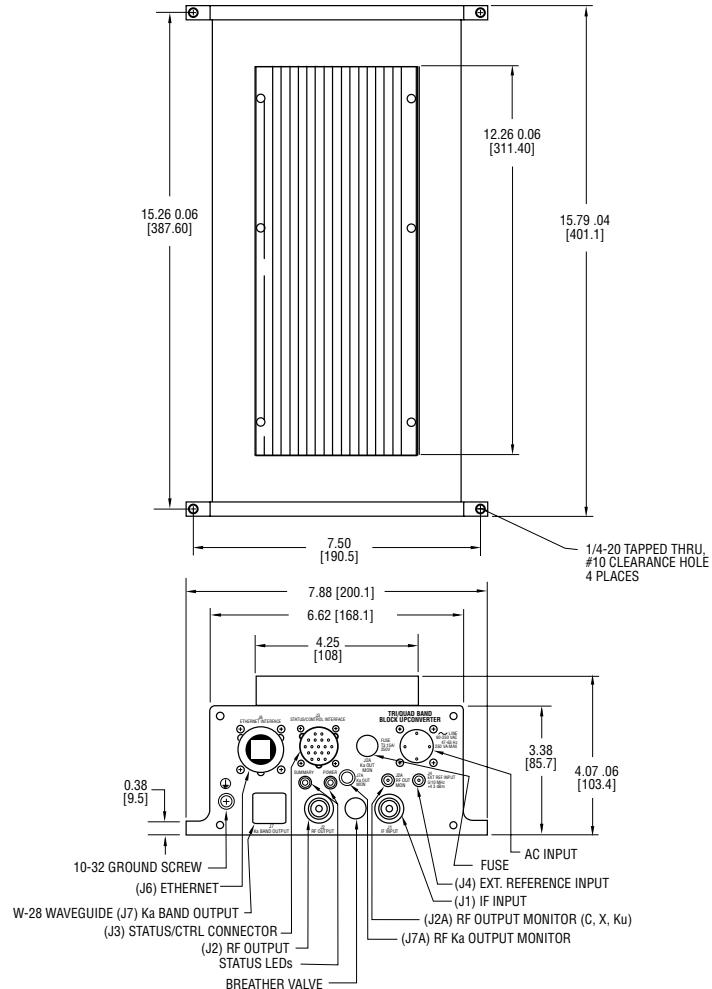
Note: Dimensions shown are in inches and those shown in brackets [ ] are in millimeters.
