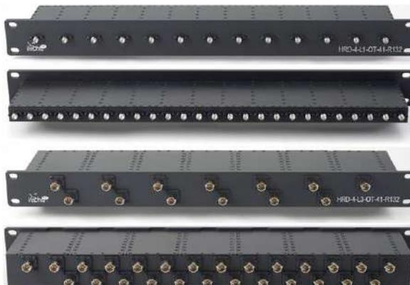
The ViaLiteHD RF splitters have been designed specifically to save space in a 19" rack deployment and in the ViaLite 19" chassis by negating the need to have a splitter card installed. With enough capacity to locally split the output from a full 19" chassis, the splitters are ideal for L-Band redundancy applications. The solution comes in two types - 50 & 75 Ohm - which are fitted with either SMA or BNC connectors accordingly.
