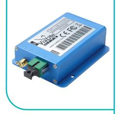
The Blue OEM Link is a small, dustproof RF over fiber module which is available in ViaLiteHD RF bands up to 4.2 GHz, in either transmitter or receiver formats. The link is available with SC or FC optical connectors and either SMA or MCX RF connectors.
