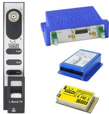
ViaLiteHD L-Band HTS fiber optic 50km links use 1550nm lasers and have been designed for the satellite industry to transport RF signals between antennas and control rooms over fiber. Due to the very wide dynamic range the same link can be used in both the transmit and receive paths.
