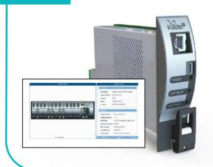
The ViaLiteHD HRC-3 rack card can be installed into the standard ViaLiteHD 19" rack shelf to monitor, log and raise alarms when events occur. The HRC-3 card utilizes SNMP protocol to communicate over Ethernet with the Horizons software package. If required, direct management of the HRC-3 is possible via a web browser, serial or CLI connections.
