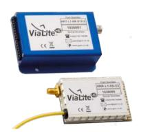
ViaLiteHD fibre optic links are available as rack mounted cards, small form factor modules and Edge OEM modules.
