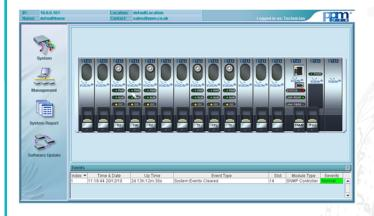
The built-in graphical user interface can be accessed from any standard web browser using the IP address of the SNMP network monitoring module.
