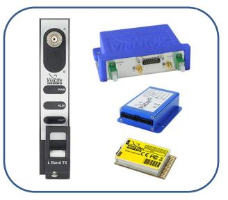
**ViaLiteHD** L-Band HTS fiber optic links have been designed for the satellite industry to transport RF signals between antennas and control rooms over fiber. Due to the very wide dynamic range, the same link can be used in both the transmit and receive paths. This dynamic range allows High Throughput Satellite (HTS) transponder bandwidths of 500, 800 or even 1500 MHz to be transported, as well as multiple standard 36 MHz transponders.
