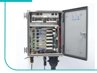
The ViaLiteHD Satcom6 weatherproof outdoor enclosure is designed to mount on or near an antenna. The enclosure accepts up to six ViaLiteHD RF or support modules including splitter and switch modules to allow for full redundancy.
