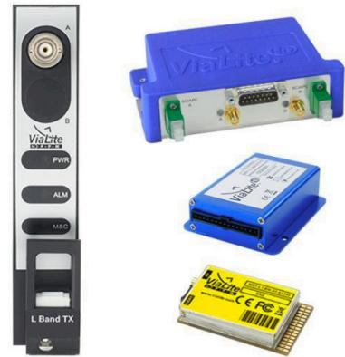
ViaLiteHD L-Band HTS fiber optic 50 km links use 1550 nm lasers and have been designed for the satellite industry to transport RF signals between antennas and control rooms over fiber. Due to the very wide dynamic range the same link can be used in both the transmit and receive paths. This dynamic range allows High Throughput Satellite (HTS) transponder bandwidths of 500, 800 or even 1500 MHz to be transported, as well as multiple standard 36 MHz transponders.
