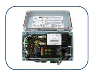
The *ViaLiteHD* ODE-MINI is a versatile enclosure designed for compact locations. The enclosure is cast aluminium and has an IP65 ingress protection rating. It is typically installed on a rooftop or antenna hub where RF and other services are transmitted over optical fiber to a remote equipment room. With options for fully integrated SNMP, Mini Ethernet Switch and LNA/B power, this enclosure is class leading for its size and cost.
