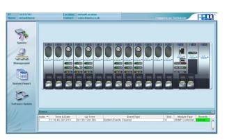
The built-in graphical user interface can be accessed from any standard web browser using the IP address of the SNMP network monitoring module.
